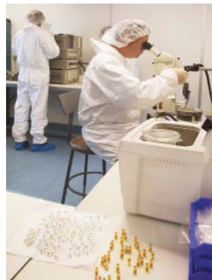
▲ Fig. 1 An HP8510 network analyser in use in the background in the Credowan clean room testing filters for the Inmarsat satellite programme.
